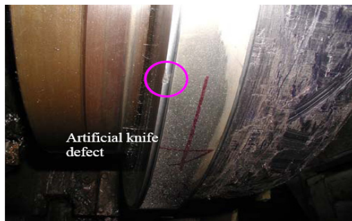
Fig. 9. An example of the artificial knife defect.
